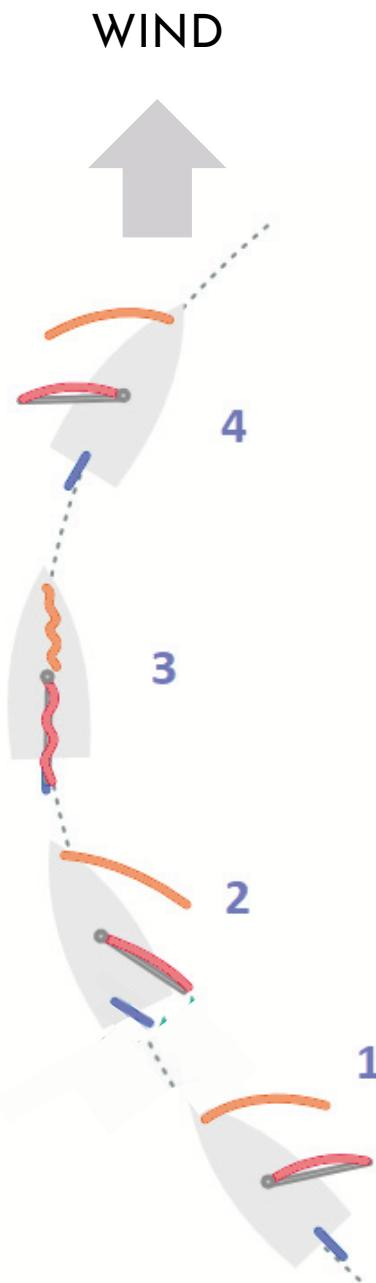
This maneuver consists of a  $60^\circ$  turn with the wind coming from behind. It starts from close hauled on port tack to close hauled starboard tack or vice versa. This is a tricky and potentially dangerous maneuver. The boom can fly from one side of the boat to the other and possibly injure someone or damage equipment. This is why we will practice the safe jibe procedure as described below.
